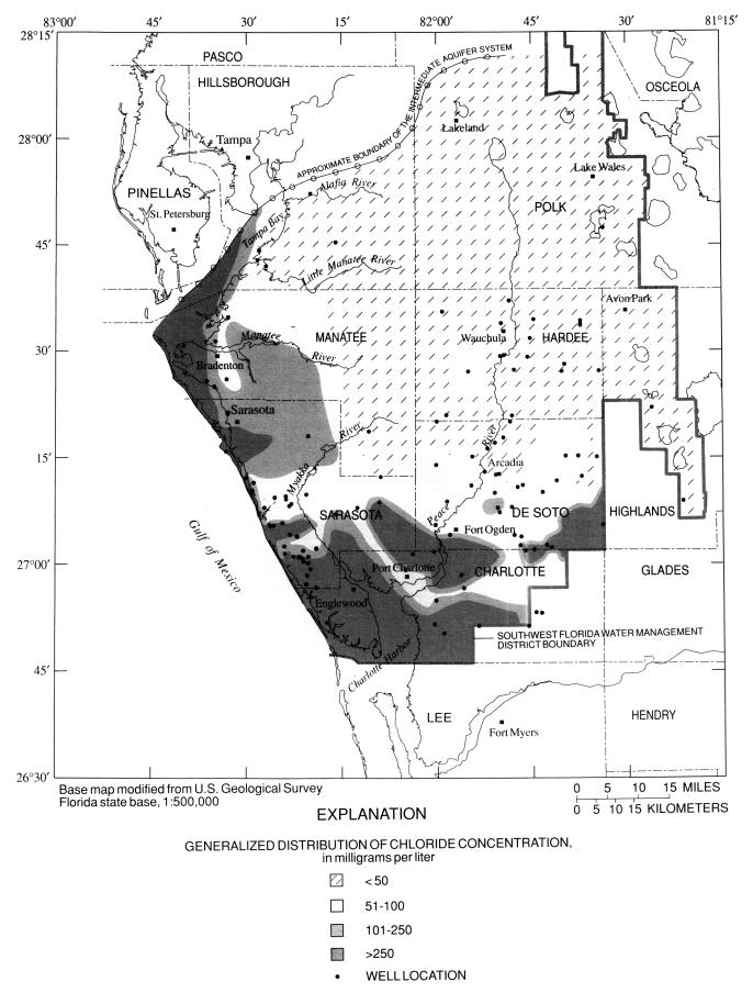
Generalized Distribution of Chloride Concentration in the Intermediate Aquifer System of West Central Florida, 1996 P. A. Metz and D. L. Brendle, USGS Water Resources Investigations Report 96-4030 (Tallahassee, FL: U. S. Geological Survey, 1996)
