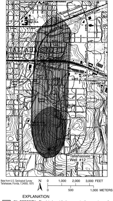
5% POROSITY—Simulated contributing area to the pumping well assuming 5% porosity, a time-of-travel of five years, and a pumping rate of 3,000 gallons per minute.
